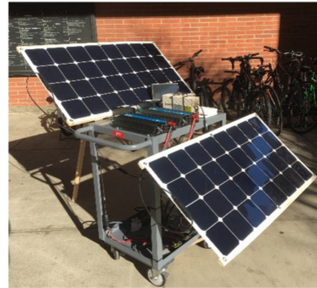
2.5 kW mobile BESS cart with 200 W PV
