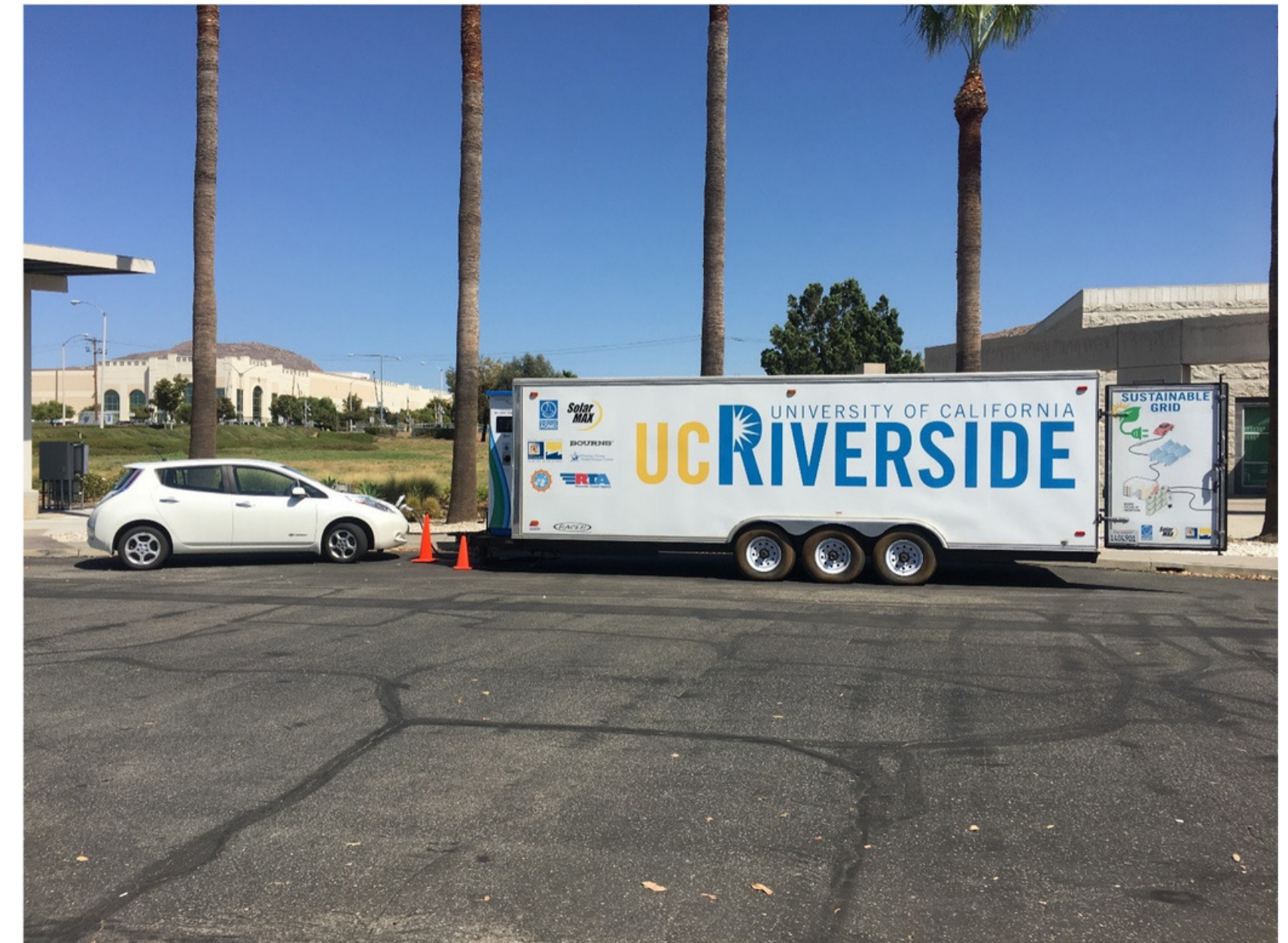
Shown in picture: Electric Vehicle supplying power to the storage bank (inside trailer) which is connected to the building microgrid
